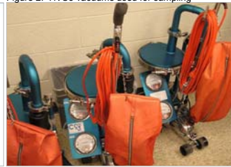
Figure 2: HVS3 vacuums used for sampling
