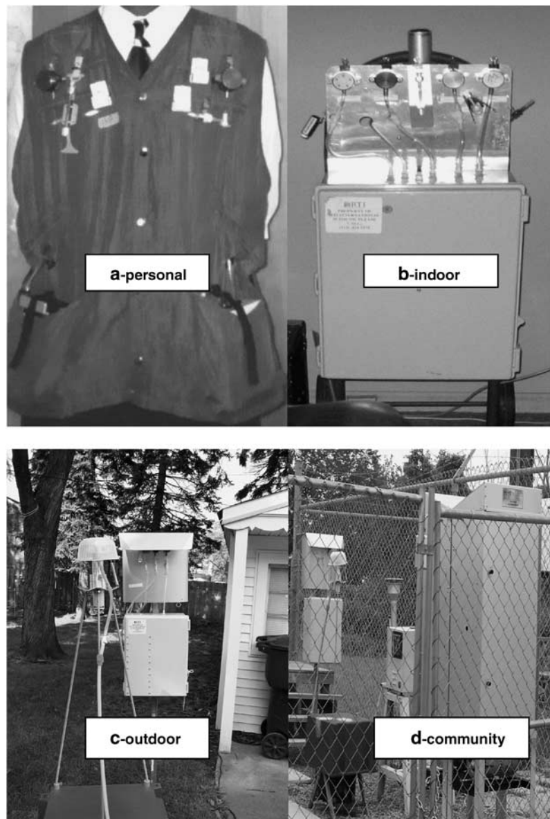
Figure 2. (a–d) Personal monitoring (a) was performed using a nylon vest with active and passive monitors positioned in the breathing zone. Residential indoor (b) and outdoor monitors (c) deployed the same equipment with the exception of weather shielding. Community monitoring (d) was conducted at a State of Michigan air monitoring site located at Allen Park.
